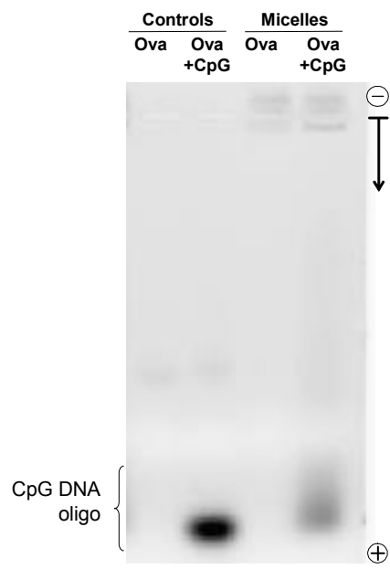
Figure 2.6. Agarose gel of SPDP-Ova/CpG micelles, prepared with 0.5 mg/mL FITC-Ova-SPDP, 0.5 mg/mL CpG DNA, and 10 mg/mL PEG-poly(Lys-Thio-Pyridyl).
